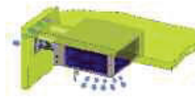
HPS in free cooling mode: use of external fresh air to maximise the energy saving
